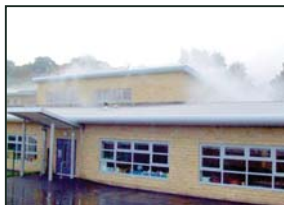
Full building smoke test
